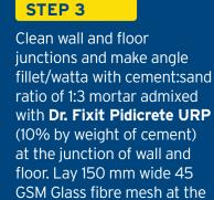
angle fillet portion in wet condition over the first coat.
